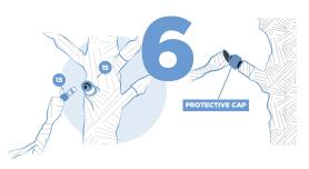
Plug the male/female electrical connectors and screw the protective cap over the connections to ensure a watertight seal.
