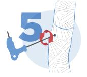
Using Allen key secure the trunk with grub screw.
