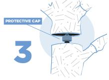
Screw the protective cap over the connections to ensure a watertight seal.
