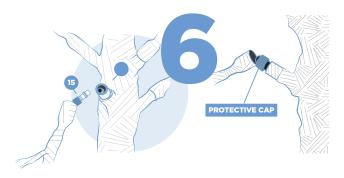
Plug the male/female electrical connectors and screw the protective cap over the connections to ensure a watertight seal.
