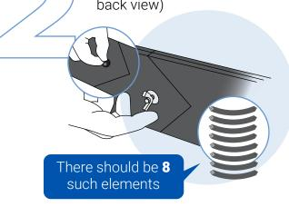
Lay out the parts, giving them the final shape of the Arch and connect with a bolt and screw. WARNING! The square cut is the facade.
